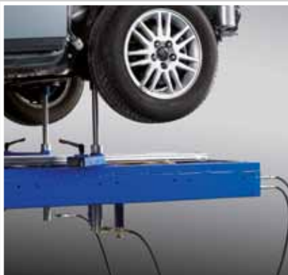
Efficient vehicle mounting with hydraulic pillar jacks
