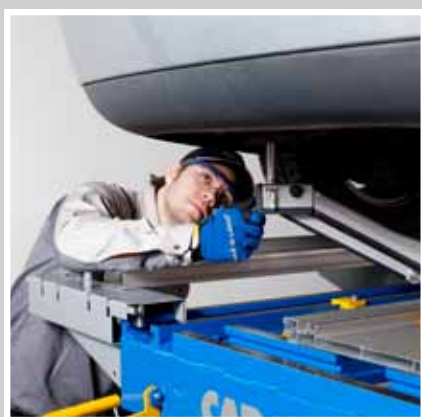
Quick diagnosis of structural damage with the vehicle supported on its wheels or in a clamped position
